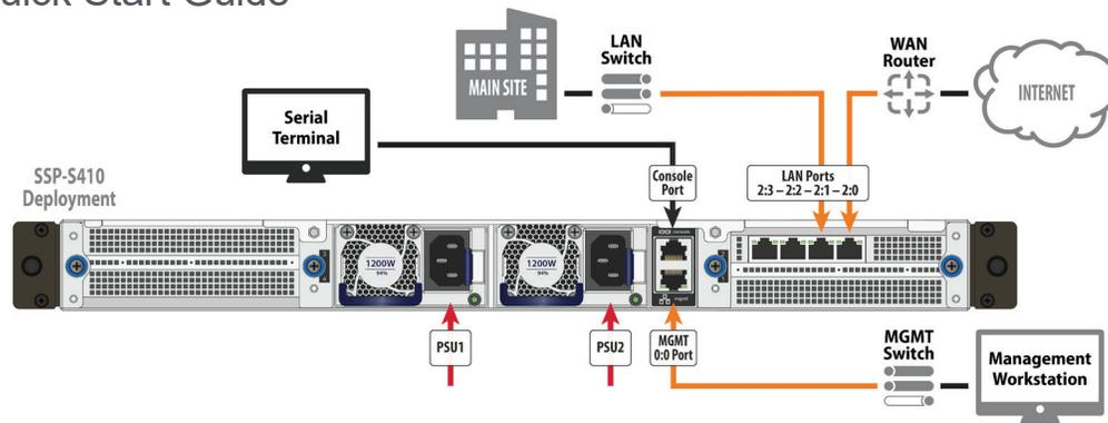
To begin using your Symantec Security Platform (SSP) appliance, complete the following steps in order. For additional instructions, including safety information, see the SSP-S410 and ISG guides, available at: [techdocs.broadcom.com](http://techdocs.broadcom.com)
